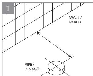
Make sure the floor drain pipe hole center, remark cross on the floor to be sure that aligning the toilet outlet hole to floor drain pipe.
