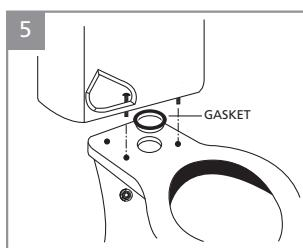
Install the gasket, then place tank over bowl and fix it with washers and nuts.
