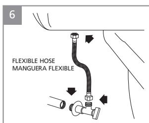
Connect the sink water inlet piping to the inlet angle valve.
