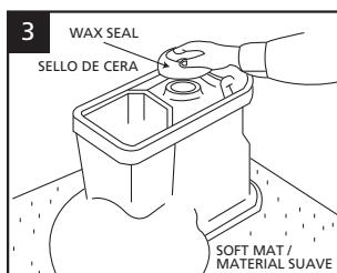
Put the toilet on a soft mat (prevent the surface of the toilet scratching). Take the new wax ring to be sure that it fits over the floor flange and fix it. Also check the sewer whether is
