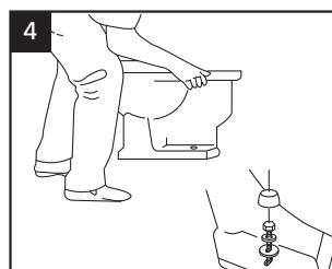
Carefully align the toilet to the hole on floor, adjust toilet until balance. Fix toilet by installing expansion bolts through toilet screw holes. Mildew proof silicon need to use on the connect place between toilet and floor.
